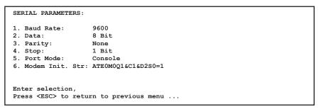
Figure 5.6: Serial Parameters Menu - Text Interface
