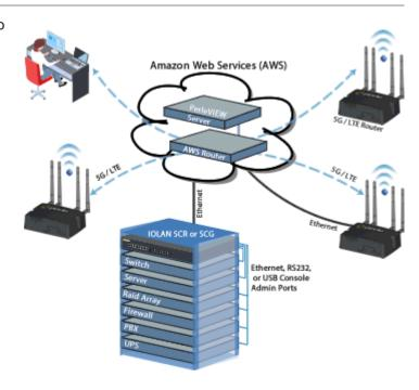
Management ports through Active Standby or Dual Network Access modes. Virtual Router Redundancy Protocol (VRRPv3) enables a group of devices to form a single virtual device to provide network redundancy. The dual AC power supply ensures that console management is available even if the primary AC power source fails. And, protection against electrostatic discharges and power surges is provided with robust 15Kv ESD protection circuitry on each console port.
