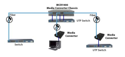
Fast Ethernet UTP Switch to UTP Switch
