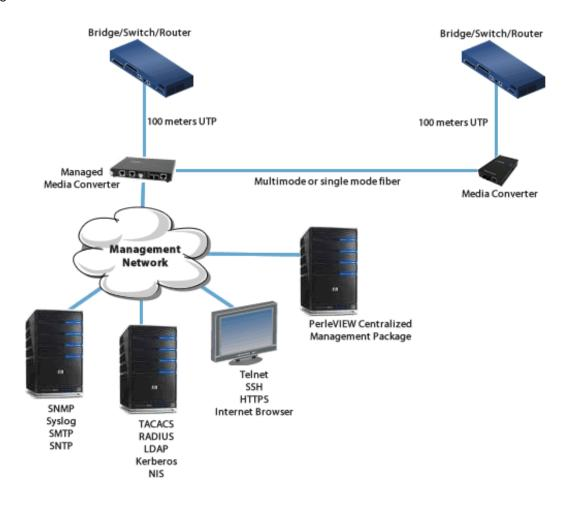
10/100 - Extend Network between Ethernet Hubs
