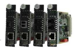
Installed in a high density Perle Media Converter Chassis, Perle's line of feature rich Managed 10/100 Rate Converting to Fiber Media Converters transparently connect 10/100 Ethernet to fiber. Our 10/100 converters provide an economical path to extend the distance of an existing network, the life of non-fiber based equipment, or the distance between two devices.
