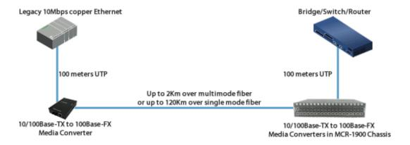
10/100 - Extend Network between Half-Duplex Hubs
