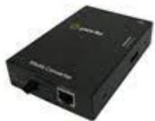
**S-100-M1ST2D - Fast Ethernet Media Converter.** 100Base-TX (RJ-45) [100 m/328 ft.] to 100Base-BX 1550nm TX / 1310nm RX single strand fiber, multimode (ST) [2 km/1.2 miles]
