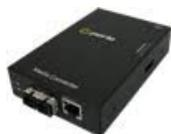
**S-100-M2SC2 - Fast Ethernet Stand-Alone Media Converter.** 100Base-TX (RJ-45) [100 m/328 ft.] to 100Base-FX 1310nm multimode (SC) [2 km/1.2 miles]
