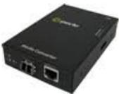
**S-100-S2LC80 - Fast Ethernet Stand-Alone Media Converter.** 100Base-TX (RJ-45) [100 m/328 ft.] to 100Base-ZX 1550nm single mode (LC) [80 km/49.7 miles]
