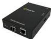
**S-100-S2LC20 - Fast Ethernet Stand-Alone Media Converter.** 100Base-TX (RJ-45) [100 m/328 ft.] to 100Base-LX 1310nm single mode (LC) [20 km/12.4 miles]
