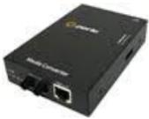
**S-100-S2ST80 - Fast Ethernet Stand-Alone Media Converter.** 100Base-TX (RJ-45) [100 m/328 ft.] to 100Base-ZX 1550nm single mode (ST) [80 km/49.7 miles]
