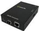
**S-100-S2LC40 - Fast Ethernet Stand-Alone Media Converter.** 100Base-TX (RJ-45) [100 m/328 ft.] to 100Base-EX 1310nm single mode (LC) [40 km/24.9 miles]
