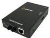
**S-100-S2ST40 - Fast Ethernet Stand-Alone Media Converter.** 100Base-TX (RJ-45) [100 m/328 ft.] to 100Base-EX 1310nm single mode (ST) [40 km/24.9 miles]
