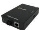
**S-1000-S1SC10U - Gigabit Ethernet Stand-Alone Media Converter.** 1000Base-T (RJ-45) [100 m/328 ft.] to 1000Base-BX 1310nm TX / 1490nm RX single strand single mode (SC) [10 km/6.2 miles]
