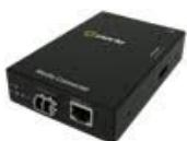
**S-1000-S2LC10 - Gigabit Ethernet Stand-Alone Media Converter.** 1000Base-T (RJ-45) [100 m/328 ft.] to 1000Base-LX/LH 1310 nm single mode (LC) [10 km/6.2 miles] or multimode (LC) [550 m/1804 ft.] using a mode conditioning patch cord.
