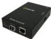
**S-1000-S2LC160 - Gigabit Ethernet Stand-Alone Media Converter.** 1000Base-T (RJ-45) [100 m/328 ft.] to 1000Base-ZX 1550 nm single mode (LC) [160 km/100 miles]
