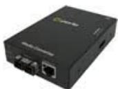
**S-1000-M2SC05 - Gigabit Ethernet Stand-Alone Media Converter.** 1000Base-T (RJ-45) [100 m/328 ft.] to 1000Base-SX 850nm multimode (SC) [550 m/1804 ft.]
