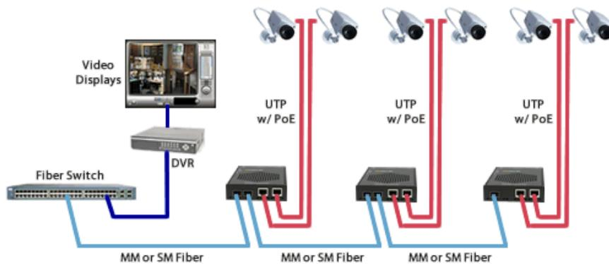
A second option is to have redundant fiber links for installations requiring fiber facility protection. There is an active fiber port and a protection fiber port that can support a fiber failure switchover of less than 50 milliseconds. The Hi-PoE media converter supplies power to the camera, and has power protection from an Uninterruptible Power Supply (UPS) battery back-up. In the event of a fiber cut and a loss of power, the camera continues to send data on the protection link.
