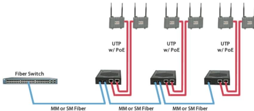
A second option is to have redundant fiber links for installations requiring fiber facility protection. There is an active fiber port and a protection fiber port that can support a fiber failure switchover of less than 50 milliseconds. The PoE+ media converter supplies power to the camera, and has power protection from an Uninterruptible Power Supply (UPS) battery back-up. In the event of a fiber cut and a loss of power, the camera continues to send data on the protection link.
