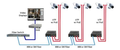
A second option is to have redundant fiber links for installations requiring fiber facility protection. There is an active fiber port and a protection fiber port that can support a fiber failure switchover of less than 50 milliseconds. The Hi-PoE media converter supplies power to the camera, and has power protection from an Uninterruptible Power Supply (UPS) battery back-up. In the event of a fiber cut and a loss of power, the camera continues to send data on the protection link.
