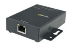
When you need to extend Ethernet services beyond the general IEEE 802.3 limits of 100m / 328ft, and new fiber cabling is cost prohibitive, the eR-S1110 Ethernet Repeater is the perfect solution. Transparently extend 10/100/1000 Ethernet connections across twisted pair (CAT5/6/7) to extend your network reach an additional 100m (328ft).
