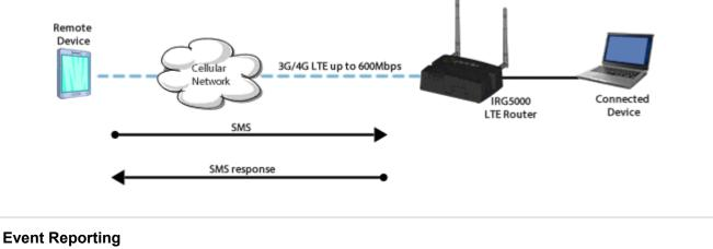
The IRG5500 Router can be configured to generate reports, or initiate actions, based on specified events. These events can be generated internally, or externally by devices attached to the IRG5500 Serial RS232, RS485, or digital inputs.
