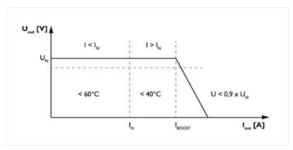
high switch-on currents of capacitive loads have to be absorbed without voltage dips.
