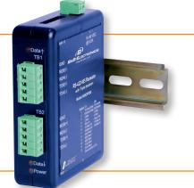
The 4850PDRI isolated RS-422/485 repeater is designed for rugged industrial environments. It is UL listed and certified for use in Class 1/ Division 2 locations. Powerful optical isolation on both data ports protects your equipment and data from damaging ground loops and surges. Additional isolation on the power supply circuits add a third degree of protection.
