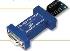
These port-powered, two channel converters allow your computer to communicate longer distances by converting TD and RD RS-232 lines to RS-485 signals. RS-485 also provides multi-drop capability.
