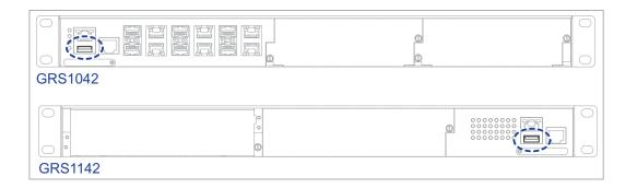
The USB interface allows you to connect the AutoConfiguration Adapter ACA22 storage medium. This is used for saving/loading the configuration data and diagnostic information, and for loading the software. See "Accessories" on page 71.
