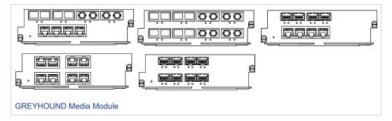
You have the option to select either 1 or 2 media modules. By using a media module, you obtain up to 8 additional Fast and/or Gigabit Ethernet ports.
