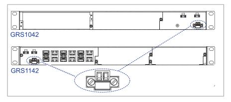
Figure 1: Signal contact: 2-pin terminal block with screw locking
