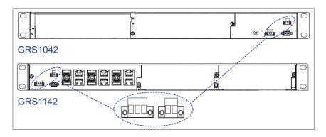
via one 2-pin and one 3-pin terminal block Device variants with characteristic value HL
