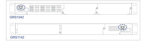
A serial interface is provided on the RJ45 socket (V.24 interface) for the local connection of an external management station (VT100 terminal or PC with corresponding terminal emulation). This enables you to set up a connection to the Command Line Interface (CLI) and to the system monitor.
