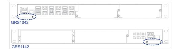
The SD card interface allows you to connect the AutoConfiguration Adapter ACA31 storage medium. This is used for saving/loading the configuration data and diagnostic information, and for loading the software. On the front of the device there is an LED display that informs you about the status of the interface.
