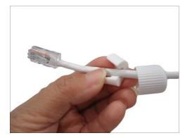
5. Insert the cable through the gland body.
