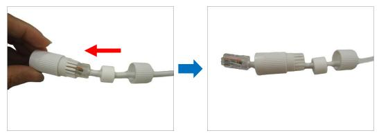
6. Push the sealing insert into the gland body.
