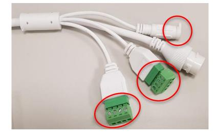
**NOTE:** If these connectors will not be used, make sure to wrap them with waterproof tape to avoid water or dust from entering the connectors.
