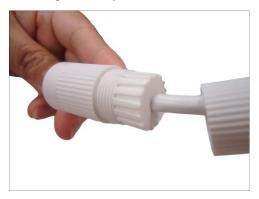
7. Connect the RJ-45 connector to the camera connector.
