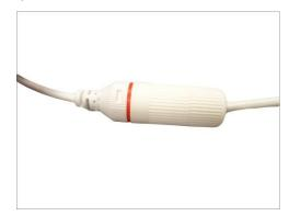
**NOTE:** Make sure the clamping nut is tightly attached to the cable gland body and the sealing insert is squeezed tightly.
