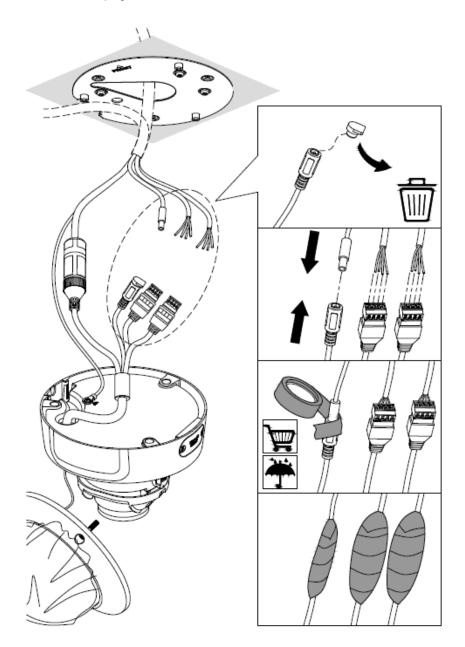
Unused cable connections must also be wrapped with waterproof tape.
