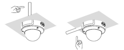
5. Mark the screw holes and cable hole (if the cable will pass through the surface) using the bundled surface mount plate as template. Then drill the necessary holes.
