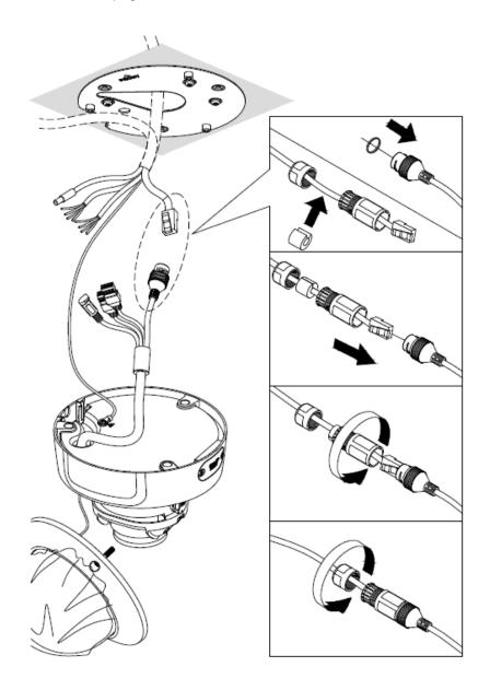
**NOTE:** If the camera will be installed outdoors or in places wherein environmental factors change drastically, make sure to waterproof the cable connections. See *How to Use the Cable Gland* on page 27.
