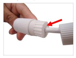
16. Connect the RJ-45 connector to the camera connector.
