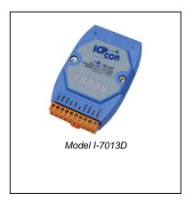
Model I-7013, I-7013D RTD Analog Input Module
