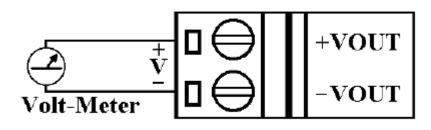
Short the current output terminal for the read-back requirement
