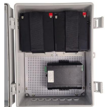
10A Solar, 30W PoE Controller Inside
