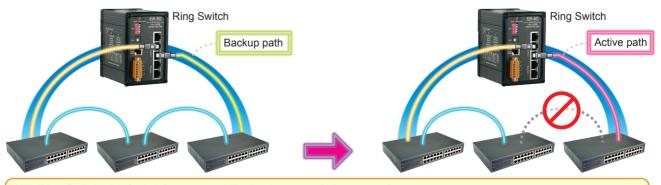
With Ring Switch, the fault-tolerant capability is given to existing network
