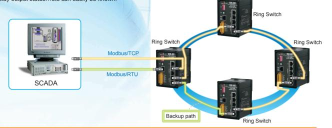
For most HMI/SCADA software tools, the availability of Modbus/TCP protocol from Ring Switch help them to monitor the status of the Ethernet LAN.
