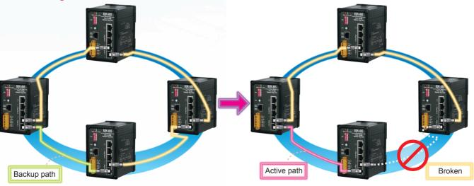
The ring topology provides an alternative network path in constant readiness. When a network node or cable segment fails, the Ring Switch instantly redirects the traffic through the alternative path of the ring.
