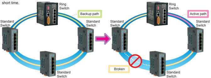
Even with only one Ring Switch in the ring network. It still provides fault-tolerance protection. Thus it becomes a very cost effective way to build your Fault-tolerant Ethernet Network.
