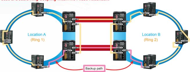
Double ring coupling with two phase redundant strenthen the coupling of 2 rings. In which ring topology, there are 2 coupling points providing redundant coupling path of 2 rings.
