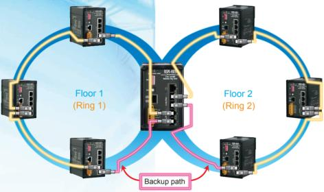
Double ring is best solution for 2-floor application scene. The 2 Ring Switch not only construct individual redundant ring for each floor but also backup each other.
