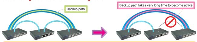
The Spanning Tree algorithm is the most universal method of provisioning multiple paths through an Ethernet network. Unfortunately, it is cumbersome and slow to converge.
