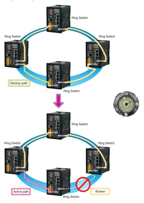
With Ring Switch, the recovering time from link loss is deterministic.
