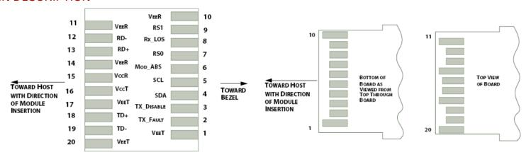
Host PCB SFP+ Pad Assignment Top View
