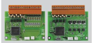
**XV107/XV107A** 8-channel Isolated Digital Input and 8-channel Isolated Digital Output Module
