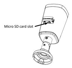
**NOTE**: Do not hot plug the memory card after it has been inserted and the power turned on, otherwise, the camera or the card might be damaged.
