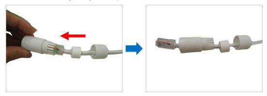
6. Push the sealing insert into the gland body.
