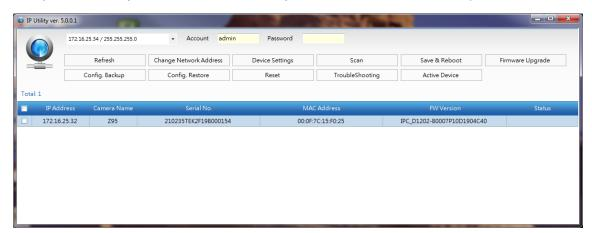
You can quickly see the camera model in the list. Double-click on the IP address to automatically launch the default browser of the PC with the IP address of the target camera filled in the address bar of the browser already.
